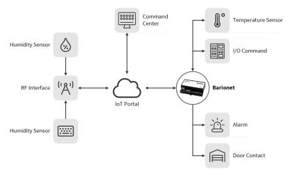
Barionet 1000 is a device server, based on Linux/Lede/OpenWRT. The device features a wide range of interfaces such as two USB, WiFi, RS322 serial port, analog and digital I/Os, Relays and Dallas 1-wire support. It is IPv4 or IPv6 capable. Supporting SNMP, Modbus and universal ASCII protocols, the Barionet device can be easily integrated into 3rd party management systems. Barix Products are developed in Switzerland and manufactured in the EU.
